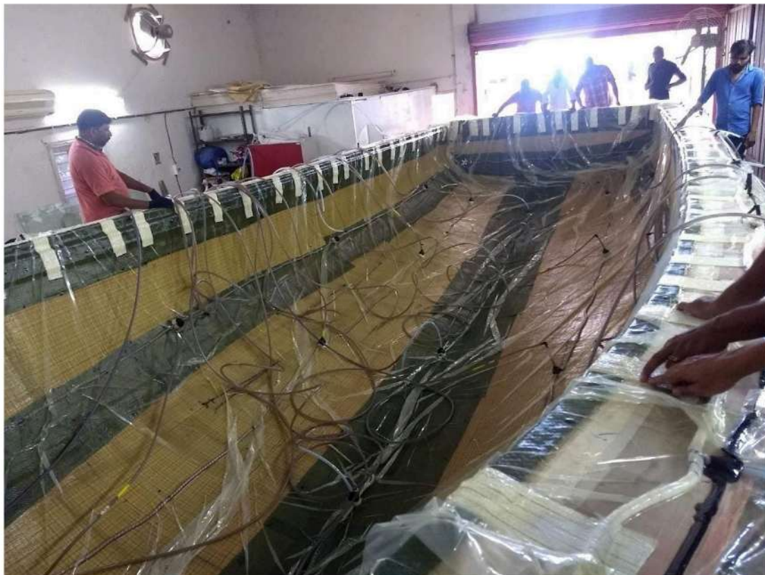
Figure 14: A series of spiral flow tubes, injection hoses, vacuum return lines, ensure controlled exothermic setting is done in the next two hours
