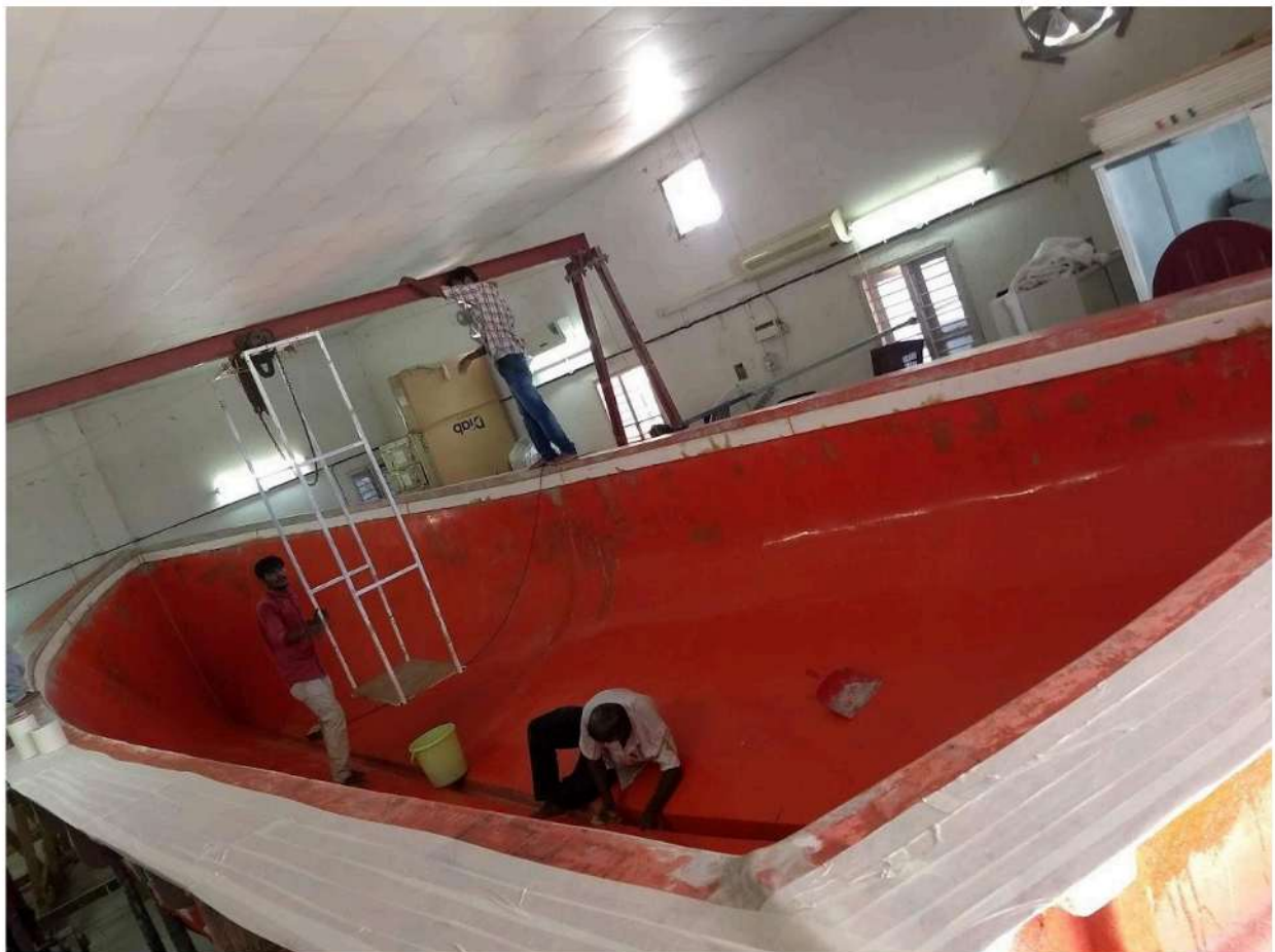
Figure 7: Surface of the female die prepared for layer layup
