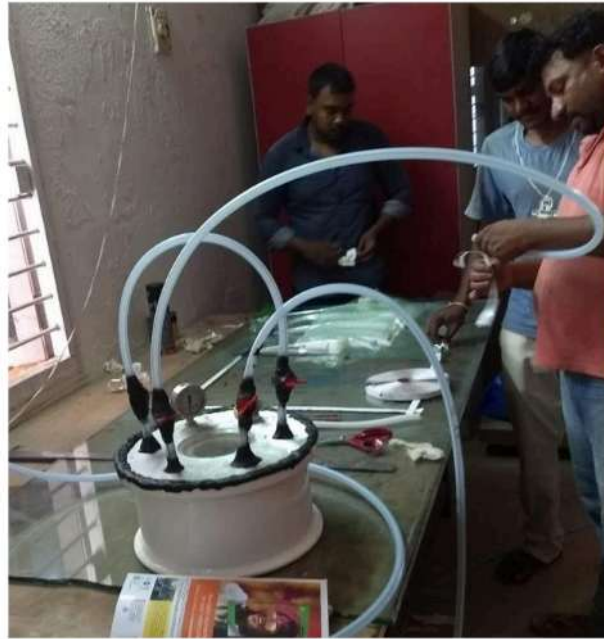
Figure 14: A series of spiral flow tubes, injection hoses, vacuum return lines, ensure controlled exothermic setting is done in the next two hours
