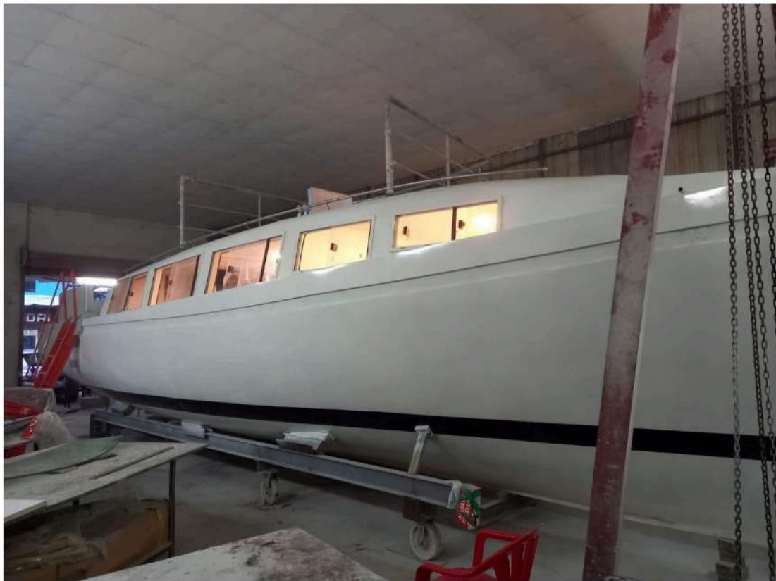
Figure 16: The final hull emerges from the die, below stern view
