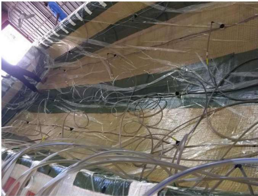
Figure 11: Quadraxial fibre layers, divinycell sandwich foam, inner quadraxial layers, peel plies, vacuum sealing
