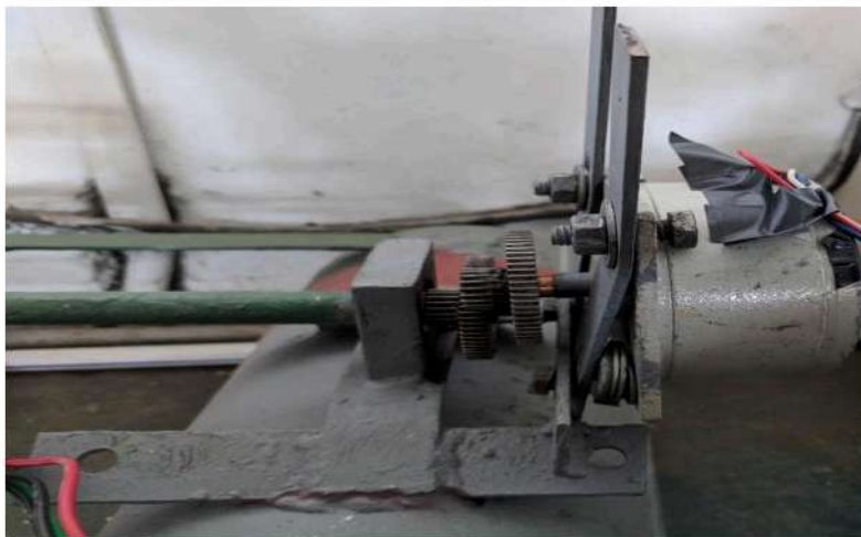
Figure.3: Shaft geared with the stepper motor
