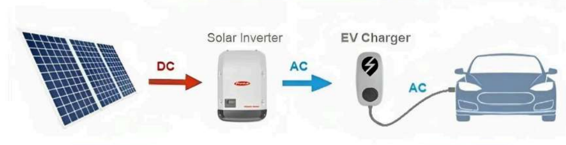
Figure 3 - A Simple Sketch of Solar Powered EV Charging Station
