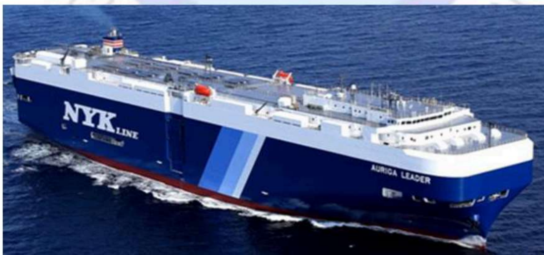
Figure 5 - Auriga Leader-world's first solar powered ship
